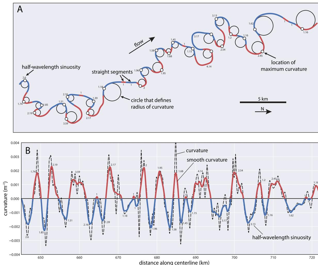
FIG. 1.—**A**) Example of a centerline segment from the Amazon Channel showing channel bends and fitted circles that define the radius of curvature. **B**) Raw and smoothed curvature calculated from the same centerline segment as in **A**. Red and blue segments correspond to channel bends with opposite signs of curvature.
